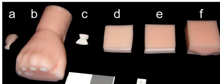
Figure 1. Gelatin tissue phantoms in variety of geometries. At left are two geometrically-accurate tissue phantoms, with a) showing a rat tibia model, and b) showing a human distal radius model. At right are four planar tissue phantoms, with c) showing a block of hydroxyapatite in gelatin as a bone layer, d) thin planar phantom, e) thick planar phantom, and f) layer simulating soft tissue.
